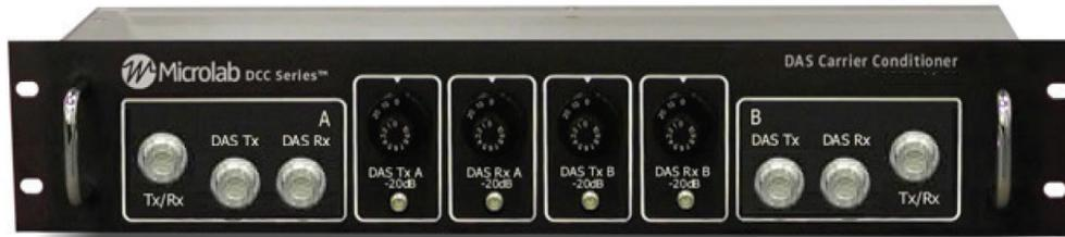
This DAS Carrier Conditioner DCC85-19-1DEFSEF3B, is designed to connect one channel of 850MHz Band and one channel of 1900MHz Band from two SISO BTS. The inputs are then separated into Uplink and Downlink for connection to a DAS system.
