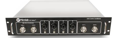
This DAS Carrier Conditioner DCC601-B42, is designed to condition and combine two channels of 2100MHz AWS1-3 SISO BTS signals. The inputs are separated into Uplink and Downlink, independently conditioned, and finally combined into a simplex output to feed into a DAS head end.
