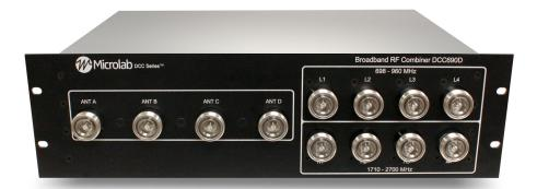
These broadband RF Combiners have been designed to meet the neutral host needs of in-building systems, with low passive inter modulation (PIM). The system combines up to 8 wireless carriers in the operating bands to 4 multiple antenna feeds or distribution cables. One quarter of each input appears on each of the four outputs, with a dissipated path loss of less than 0.5 dB.
