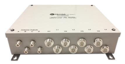
These broadband RF Combiners have been designed to meet the neutral host needs of in-building systems, with low passive intermodulation (PIM). The system combines up to 8 wireless carriers in the operating bands to 4 multiple antenna feeds or distribution cables. One quarter of each input appears on each of the four outputs, with a dissipated path loss of less than 0.5 dB.
