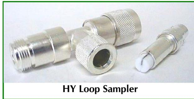
The HY probe consists of a non-directional loop, which intercepts the magnetic field in the main line and also provides a DC return in the branch line.
