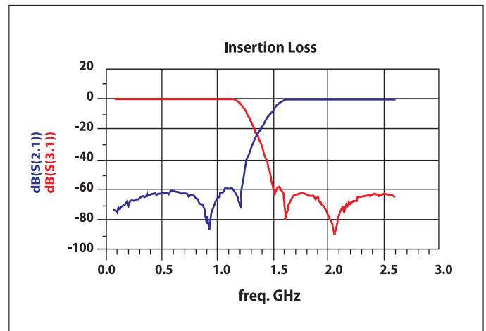
Fig 3: Insertion loss characteristics of a Microlab diplexer
