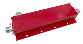
The CC-PS-x-396FN series of directional coupler is a tapered stripline design covering from 340 to 960 MHz. The units couple off a defined fraction of signal with high directivity and minimal loss. Availability in a wide range of coupling values makes this series useful in optimizing the signal distribution required in a Public Safety passive distribution network.
