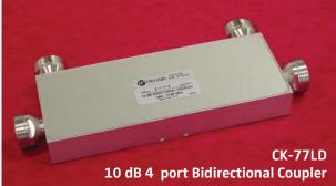
The CK-70 series, Directional Couplers, is a multi-section quarter wave, air-line design for indoor applications covering all Tetra and cellular bands, 380 to 2700 MHz and usable down to 80 MHz. Units couple off a defined fraction of signal with minimal reflections or loss.
