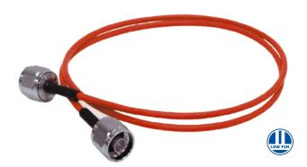
Microlab JA-PS Series coaxial cable assemblies are developed for reliability and guaranteed low PIM performance. These cables are designed with a red plenum jacket to help visually aid AHJs and building owners to identify public safety DAS networks. JA-PS cables are ideal interconnections between radios, antennas, and RF passive components
