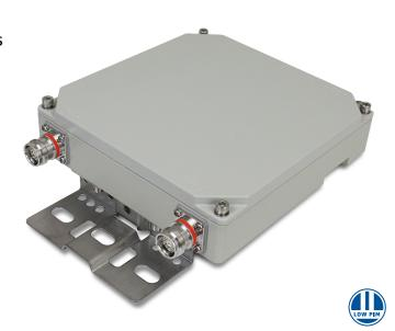
Microlab BK-2005E diplexer allows combination and separation of the signals in 1710-1735/2110-2135 MHz and 1760-1780/2160-2180 MHz commercial wireless bands. For minimum band interaction, the inputs are well isolated and have minimal insertion loss over their respective frequency bands. Attention to mechanical design ensures it guaranteed low passive intermodulation. The diplexer is designed to minimize cost and size for Small Cell & DRAN applications.
