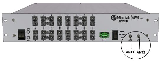
Note: DC supply to antenna ports is +5V nominal, 100mA max
