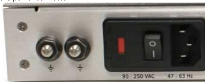
Figure 13 - Power Connection, Power Switch, Fuse holder, and Ground lugs
